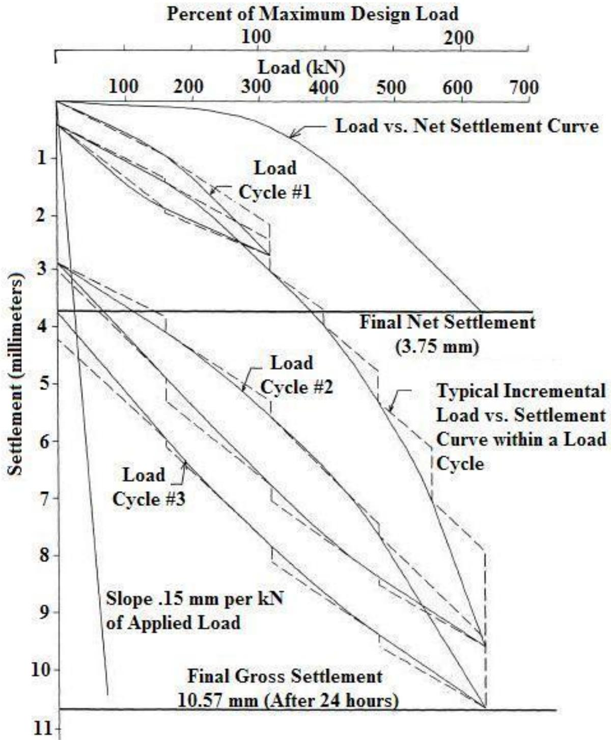
Figure 18 (b) Typical Load vs. Deflection Plot for Incremental Static Load Test
