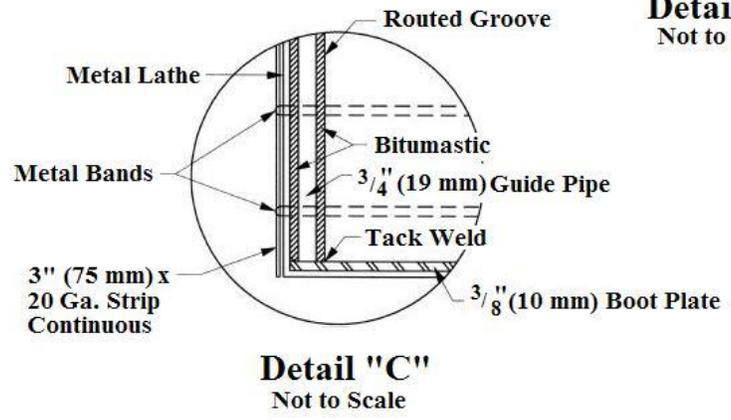
**Figure 14 Dial Support and Telltale Attachment Details for Timber Piles**
