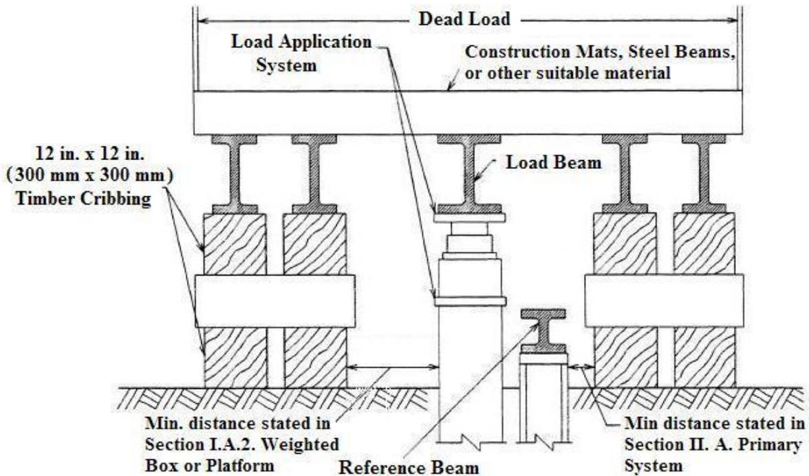
**Figure 2 Typical Setup for a Weighted Box or Platform**
