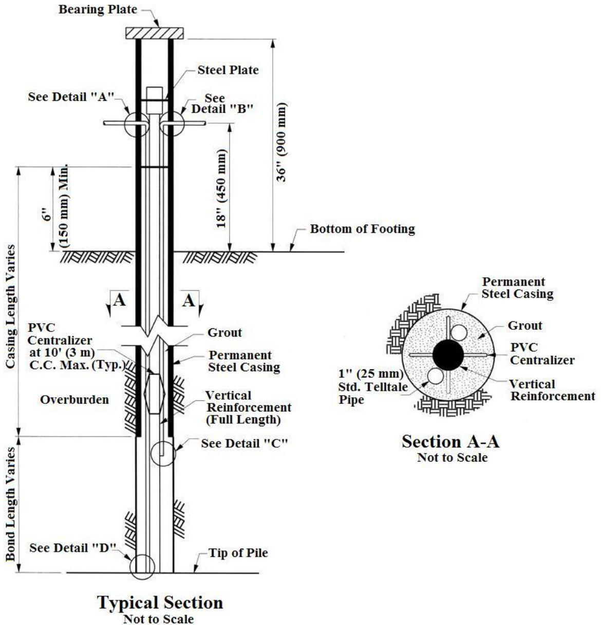
**Figure 11 Telltale Installation Details for Micropiles**
