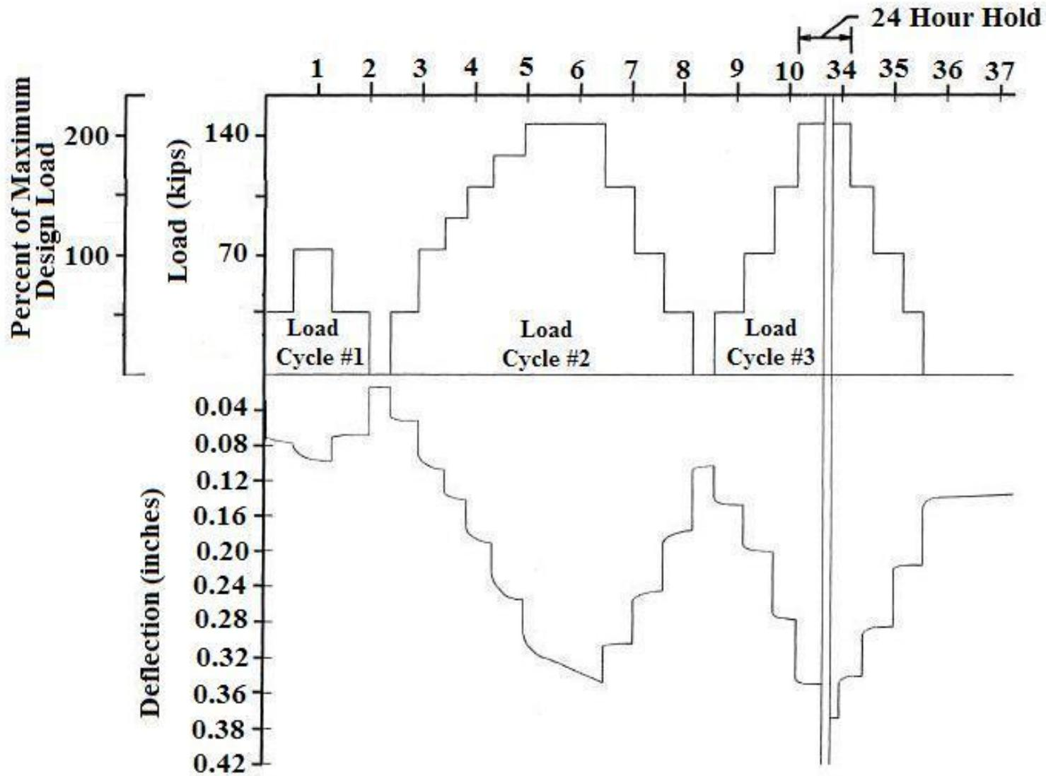
Figure 19 (a) Typical Load-Deflection vs. Time Plot for Incremental Static Load Test (*US Customary Units*)
