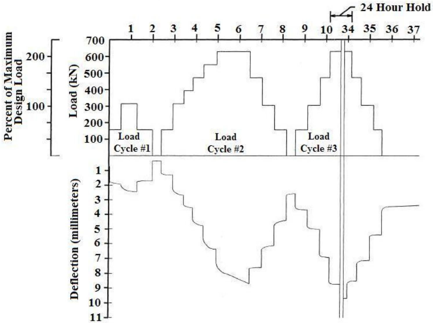
Figure 19 (b) Typical Load-Deflection vs. Time Plot for Incremental Static Load Test
