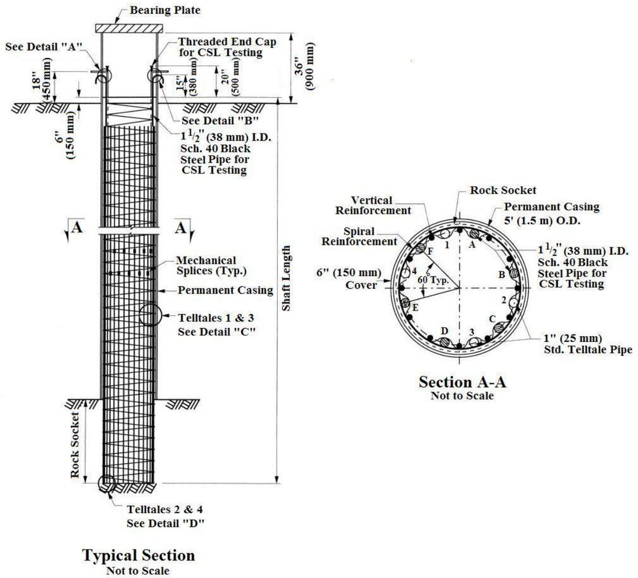
**Figure 9 Telltale Installation Details for Drilled Shafts**
