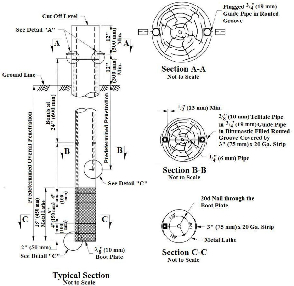
**Figure 13 Telltale Installation Details for Timber Piles**
