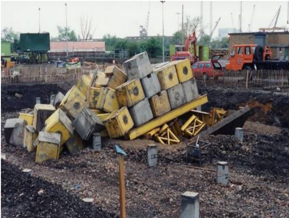
Figure 2.2 Platform bearing failure under kentledge test
