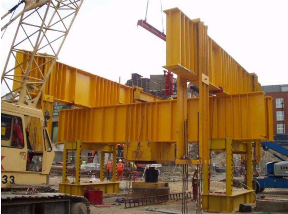
Figure 5.1 30MN reaction pile test
