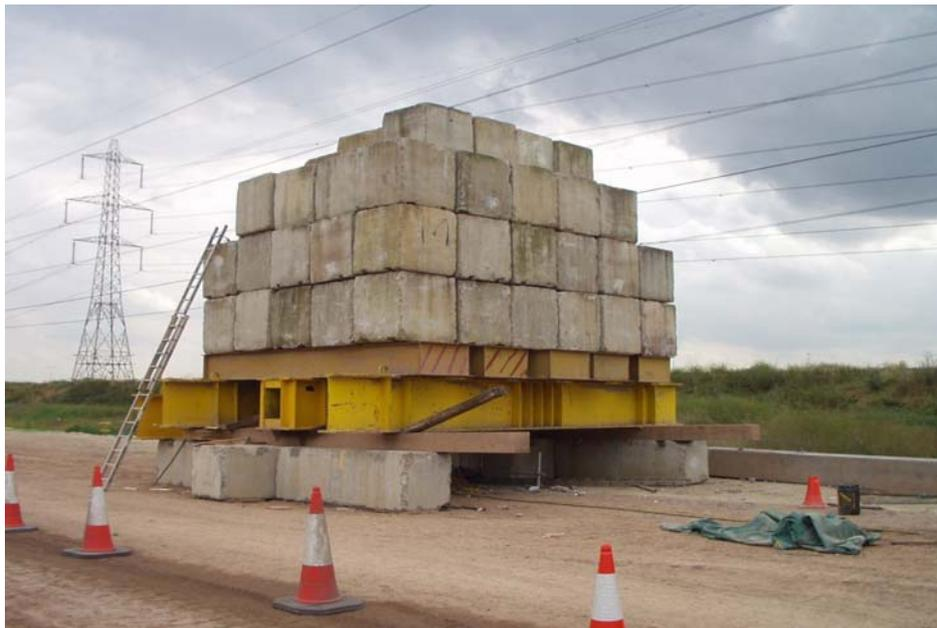
Figure 5.3 3MN kentledge test
