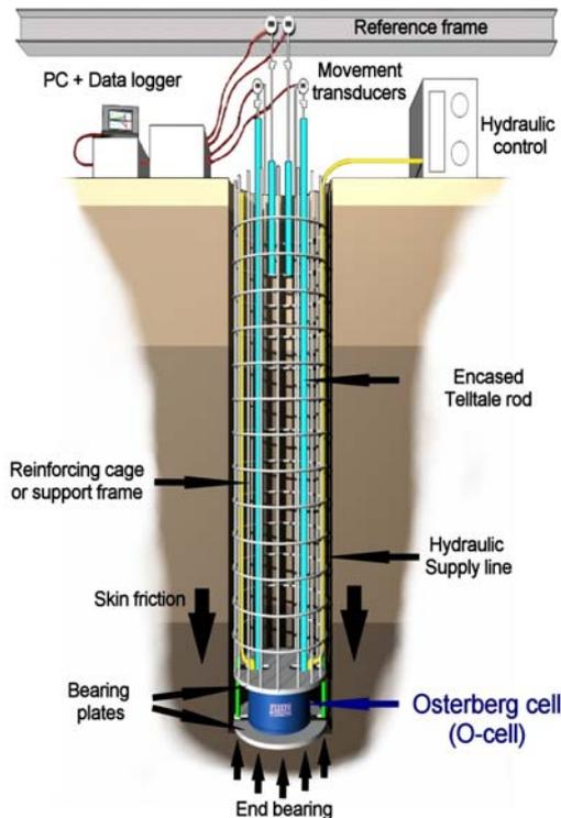
Figure 5.5 Schematic details of system
