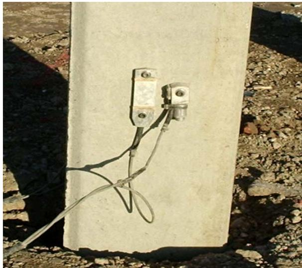
Figure 5.9 Strain gauge and accelerometer bolted to precast concrete pile
